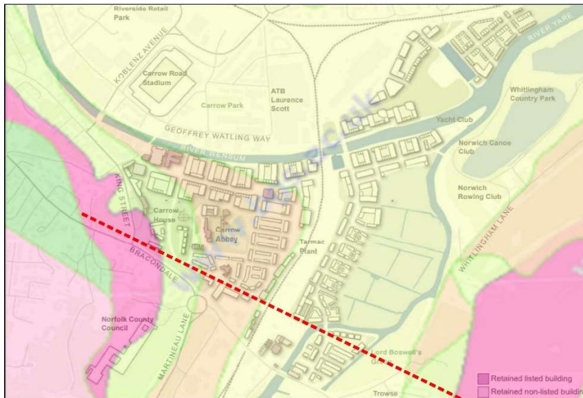
East Norwich Masterplan proposals superimposed over published geological map, with approximate line of cross section in red
