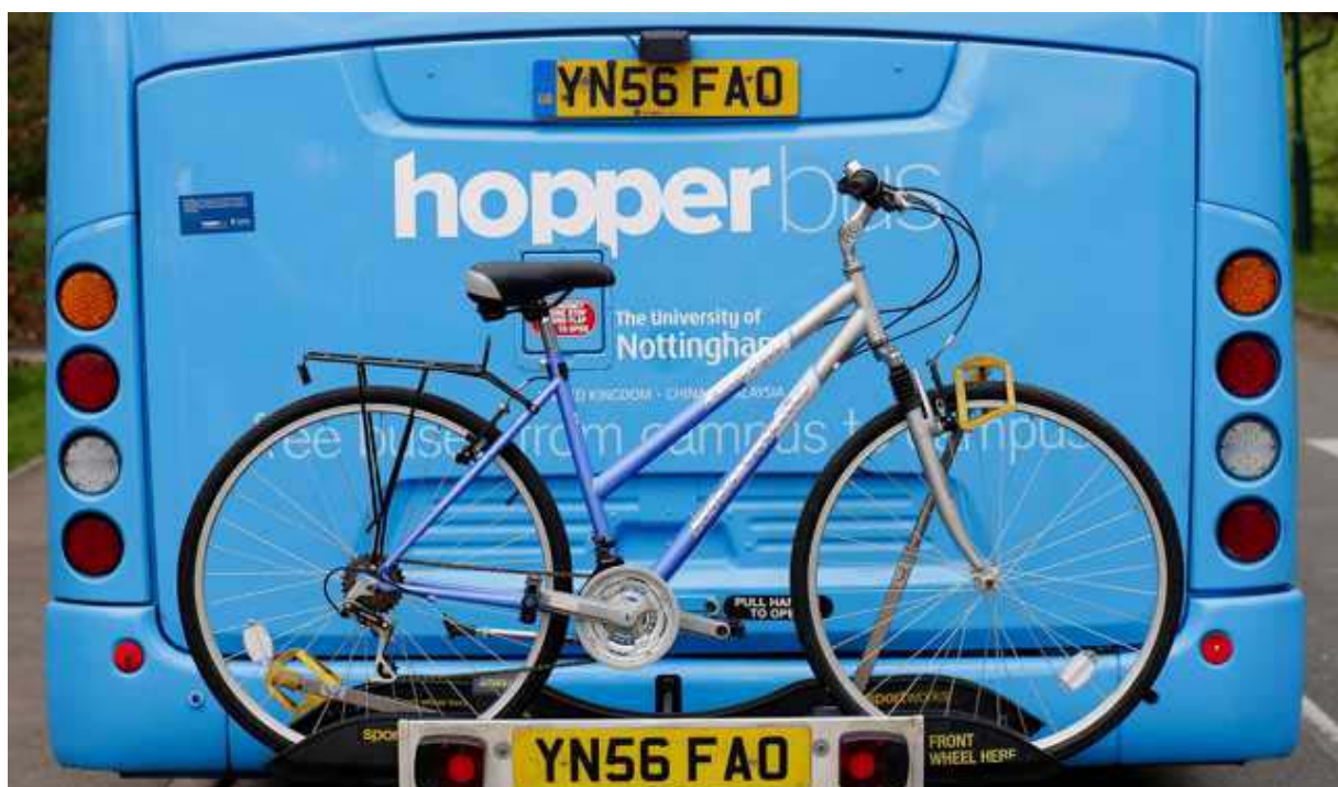
Some buses are equipped to carry one or more bikes either on the front or rear of the vehicle
